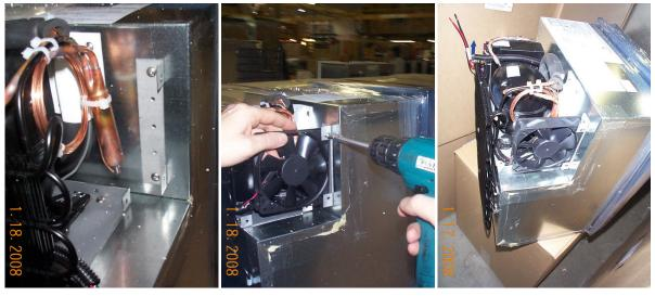
Connect the red wire to the "+", (we have provided a piggy back terminal for the DC connection) and connect the black wire to the "F" terminal
