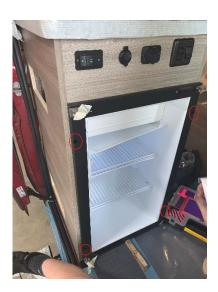
3) Remove bottom vent from galley cabinet to locate the tie down strap to the floor.
